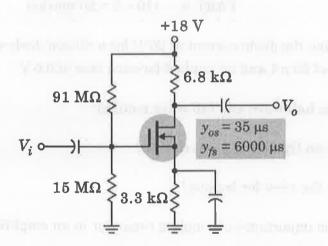
Find the output voltage  $V_o$ , for the input voltage  $V_{in} = 4$  mV.
